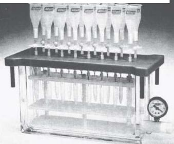
16-Port vacuum manifold for use with solid-phase extraction tubes
