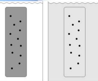
Illustration of a dialysis membrane in action.In (a) the sample solution is placed in the dialysis tube and submerged in the solvent.(b) Smaller particles pass through the membrane, but larger particles remain within the dialysis tube.
