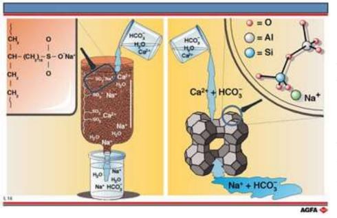
Ion exchange is a process by which ions held on a porous, essentially insoluble solid are exchanged for ions in a solution that is brought in contact with the solid. The ionexchange properties of clays and zeolites have been recognized. Synthetic ion-exchange resins were first produced in the mid-1930s and have since found widespread application in water softening, water deionization, solution purification, and ion separation.
