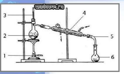
Typical equipment for a (a) simple distillation; and a (b) fractional distillation.
