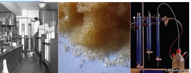
Synthetic ionexchange resins are high-molecularmass polymers that contain large numbers of an ionic functional group per molecule.
