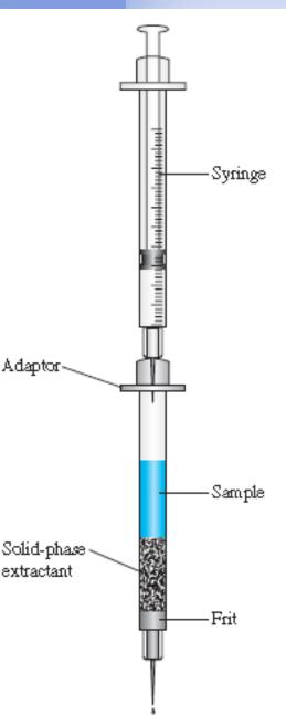
Solid-phase extraction performed in a small cartridge. The sample is placed in the cartridge and pressure is applied via a syringe plunger. Alternatively, a vacuum can be used to pull the sample through the extracting agent.
