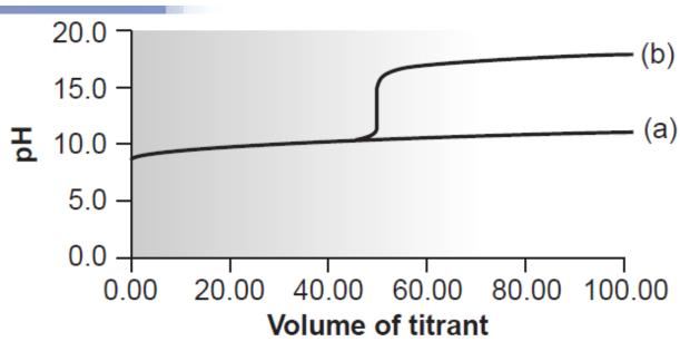
Titration curves for 50.00 mL of 0.100 M weak acid (p $K_a$ = 11) with 0.100 M NaOH in **a)** water,  $Kw = 10^{-14}$ ; and **b)** nonaqueous solvent,  $K_s = 10^{-20}$ .
